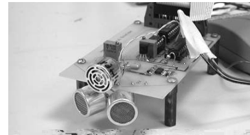
Fig. 6. Photo of the binaural sonar used in testing the LSO neuron chip. The inputs to the chip during the loud, outgoing echolocation pulse were strongly attenuated to simulate the middle-ear muscle attenuation in mammalian ears that attenuates self-generated sounds.
