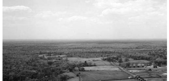
Fig. 1. Visual-horizon detection from relatively high altitude can provide valuable sensory data for flight stabilization of micro aerial vehicles, from early dawn to well after dusk.
