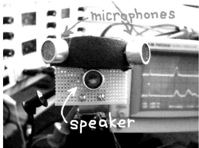
Fig. 4. Photo of the narrowband sonar front-end. The oscilloscope in the background on the right shows an example echo return from the three legs of a tripod. The sonar head is approximately 2.5'' tall and is mounted on a model airplane servo for tracking experiments (not described).
