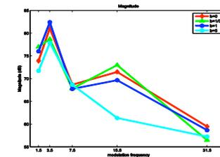
The Transfer Function is independent of bandwidth, and has the shape of a lowpass filter except for a peak near 4 Hz.
