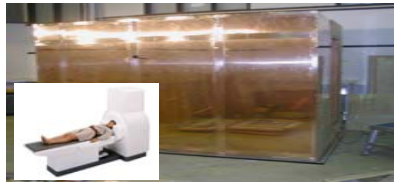
Figure 1 KIT-UMD whole head MEG system & shielded room
